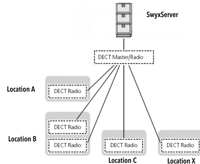
Fig. 1-4: Installation at multiple locations
