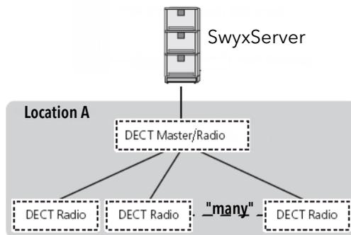
Fig. 1-3: Installation at one location
