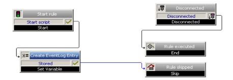
The script is entered in the "User Script" field located on the "Parameters" tab of the Start rule block. This Visual Basic Script is started if this script is called during call handling.
