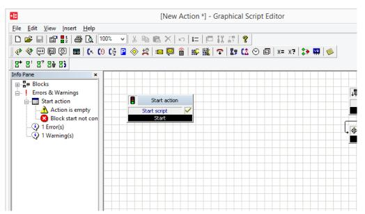
You can now position the blocks you want on the grid interface in the script window and enter the appropriate parameters. The contacts of all blocks (the input as well as the outputs) must be connected. In the Info pane you will see the messages concerning the errors and warnings. These messages provide information concerning any missing connections or parameters.
