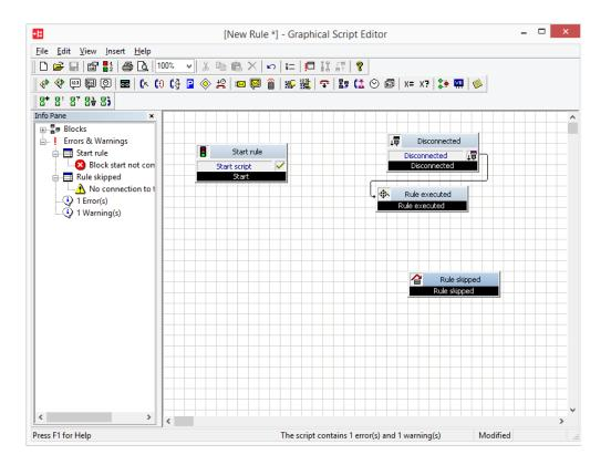
You can now position the blocks you want on the grid interface in the script window and enter the appropriate parameters. The contacts of all blocks (the input as well as the outputs) must be connected. In the Info pane you will see the messages concerning the errors and warnings. These messages provide information concerning any missing connections or parameters.
