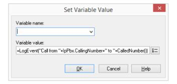
In this example, the system functions, which contain parameters for the current call (e.g. CallerNumber() and CalledNumber()), are transferred to this sub-program.
